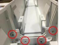
7. **[CONTINUOUS ONLY]** Reinstall module plate one by one and connect male and female disconnectors of matching colored-wires, and tuck it under the module plate.
